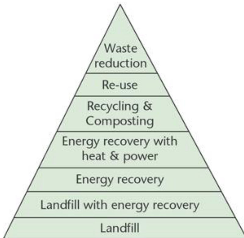
Figure 1-2: The waste management hierarchy: measures at the top of the pyramid get priority
